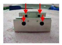
Step 5: Fix HDD box on the units with three screws
